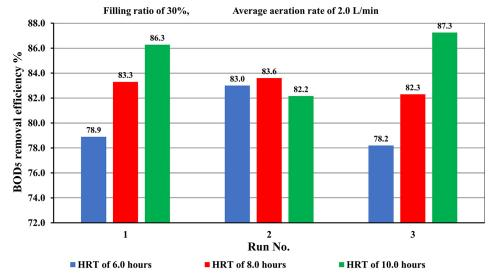
Figure 6. BOD, removal efficiency at different HRTs
