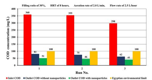
**Figure 10.** Inlet and outlet COD concentration of MBBR with and without nanoparticles compared with Egyptian environmental low limits of low 48 for year 1982
