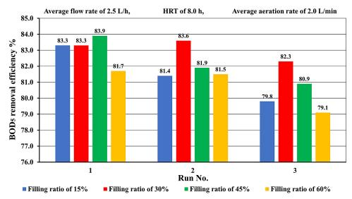
Figure 3. BOD, removal efficiency at different filling ratios
