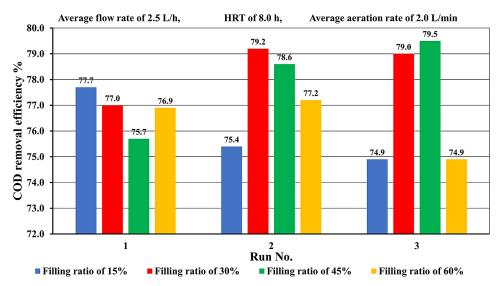
Figure 4. COD removal efficiency at different filling ratios
