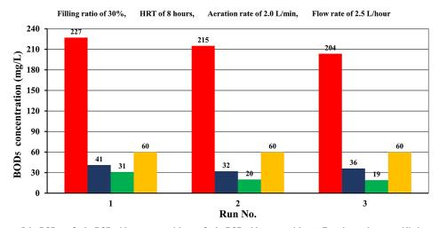
■ Inlet BOD ■ Outlet BOD without nanoparticles ■ Outlet BOD with nanoparticles ■ Egyptian environmental limit
