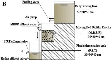
**Figure 2.** Experimental setup of MBBR system followed by settling tank in (a) a photo image, (b) a schematic diagram
