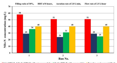
■ Inlet NH4-N ■ Outlet NH4-N without nanoparticles ■ Outlet NH4-N with nanoparticles ■ Egyptian environmental limit Figure 11. Inlet and outlet NH<sub>4</sub><sup>+</sup>-N concentration of MBBR with and without nanoparticles compared with Egyptian environmental low limits of low 48 for year 1982
