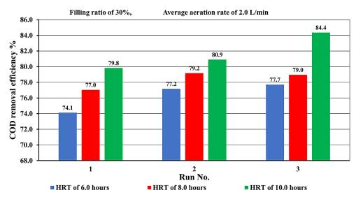
Figure 7. COD removal efficiency at different HRTs
