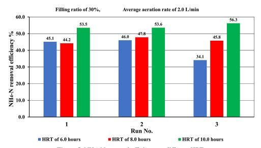
Figure 8. NH<sub>4</sub><sup>+</sup>-N removal efficiency at different HRTs
