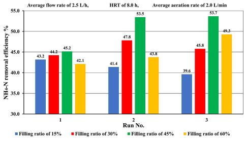
Figure 5. NH<sub>4</sub>+-N removal efficiency at different filling ratios
